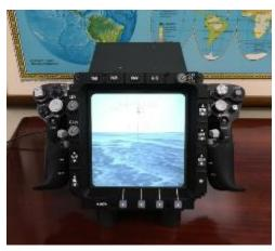
base that supports the grip assembly such that the bottom of the grip will be approximately 1" off the table surface. The LPT TEDAC Grip Assembly will report switch positions and transducer readings through a USB HID interface.
