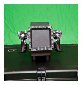
silhouette representation of the TEDAC monitor. This removable section allows for future growth to include a functional TEDAC display. The structure provides a padded base that supports the grip assembly such that the bottom of the grip will be approximately 1" off the table surface. The LPT TEDAC Grip Assembly will report switch positions and transducer readings through a USB HID interface.
